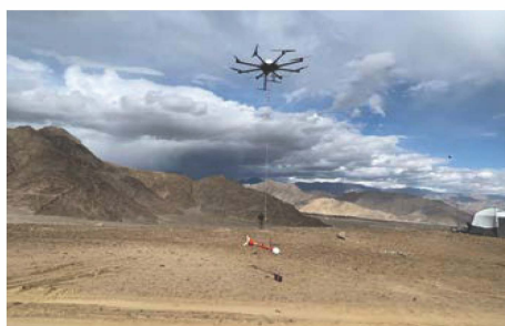
Drone based Magnetic Survey in Ladakh
